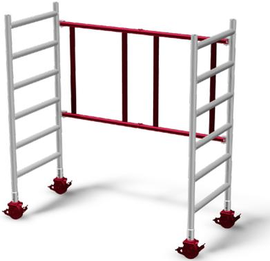
Install 4 wheels into the base of the folding frame. Once fitted unfold the frame and ensure that the back framework is locked open. Now apply the brakes to the wheels.
