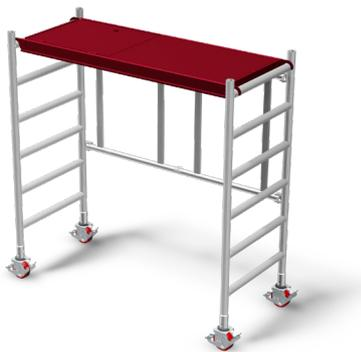
Install the wheels and lock frame open as detailed in step 1 above. Make sure the wheels are braked. Next, install the platform onto the appropriate height rung on the folding frame. Make sure the wind latches on both ends of the platform are applied.
