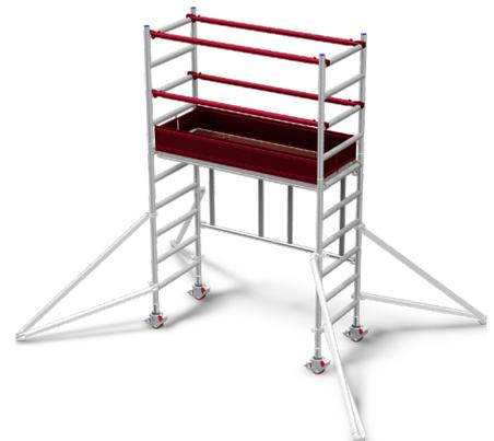
Now using the 3T method, fit the correct number of braces as specified in the component schedule to ensure that a guard rail is located on both sides of the platform at 0.5m and 1m heights. Finally fit the toeboard to the platform.
