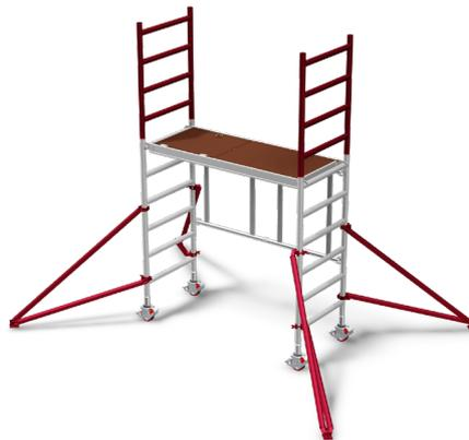
Fit into the top of the folding frame the correct extension frames as specified in the component schedule. Make sure the conical head fitting is pointing the right way so the node fits through the hole in the folding frame. Fit 4 stabilisers to the folding frame.
