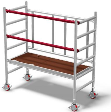
Install the platform onto the appropriate height rung on the folding frame. Make sure the wind latches on both ends of the platform are applied. Now fit 2 horizontal braces to the outside face of the frame on the 2nd and 4th rung up from the platform.
